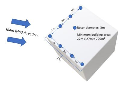
Figure 12: Exemplary building with seven installed turbines.
