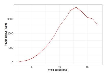
Figure 11: Power curve of the sample turbine Aeolos-V-3kW
